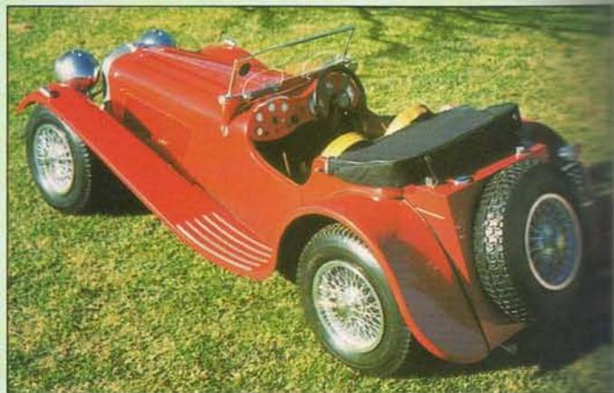
Oz-built half-scale SS 100 can travel at "fast walking pace" with the gear lever acting as forward/reverse control on the rubber belt and cog gearing. Almost everything has been made from scratch.
