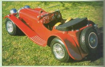
Oz-built half-scale SS 100 can travel at "fast walking pace" with the lever acting as forward/reverse control on the rubber belt and cog gearing. Almost everything has been made from scratch.
